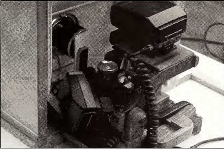
Figure 7. Relative positions of specimen staging boards and flash guns.
